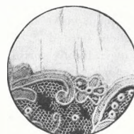
After 12 washings with an ordinary good soap—silk fibres a little out of place—lace damaged. Lustre slightly injured, color lifeless, dulled.
